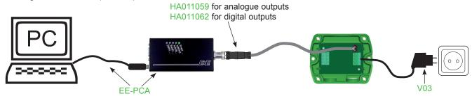
One can assign other physical quantities to the analogue outputs, change the scaling of the outputs and perform one or two point adjustment for humidity and temperature.
